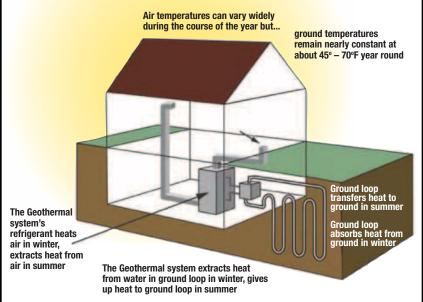
Depending on your building site, the loops can be installed either vertically (as shown) or in a horizontal orientation. With the majority of the heating and cooling capacity coming from the earth and pumped through these loops, the outside air temperature does not affect performance. So even in the cold of winter and peak summer heat, you can expect both comfort and savings on your energy bill.
